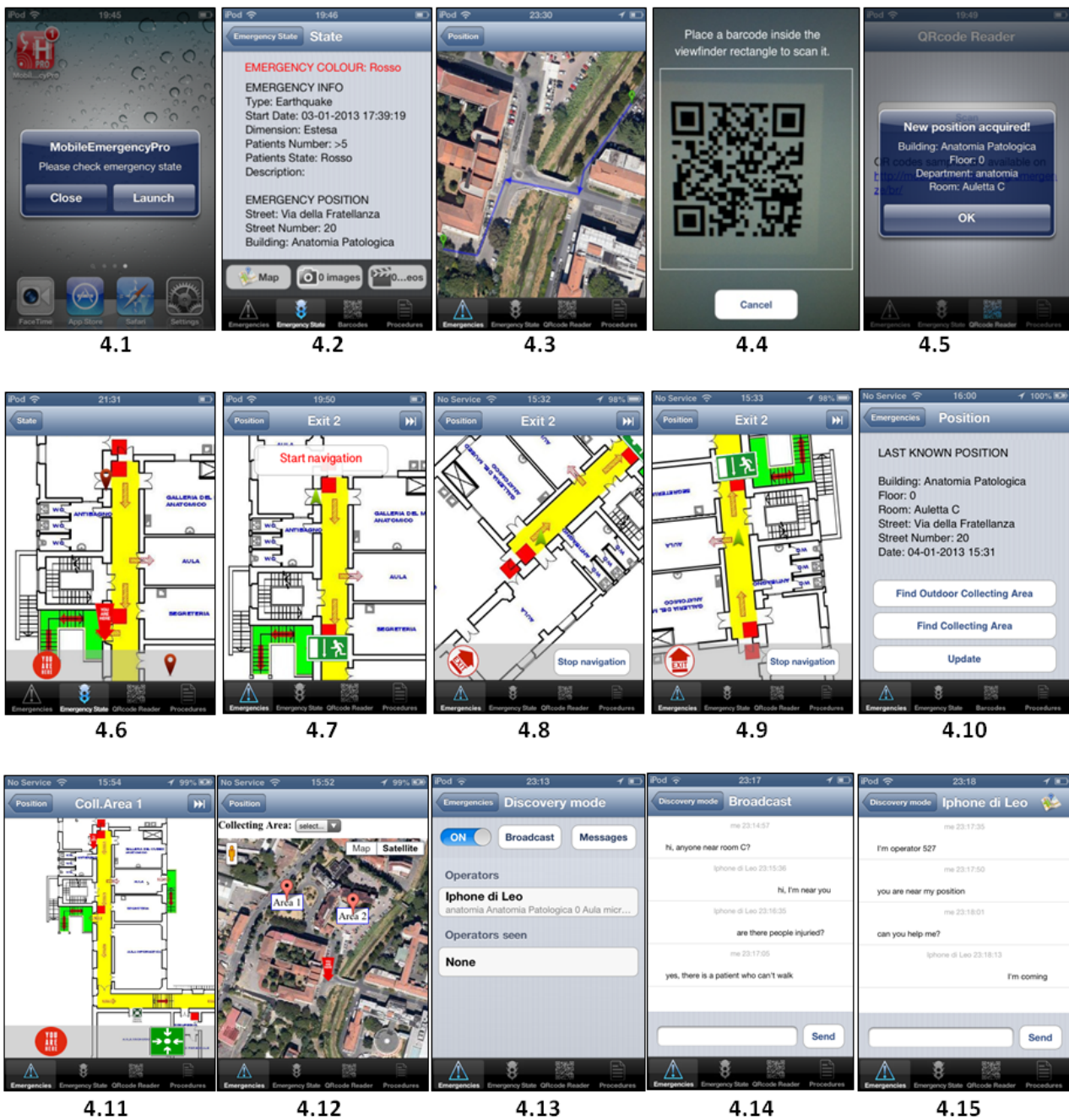
Figure 4. Scenario B: from 4.1-4.2, the emergency team reaches the emergency location. Scenario C: direct exit from (4.4-4.5) to move out (4.7-4.9). Scenario D: from emergency location (4.4-4.5) to collecting areas indoor (4.11) and outdoor (4.12). Scenario E shows some snapshots of direct discovering and chat among personnel in the emergency area (4.13-4.15).
