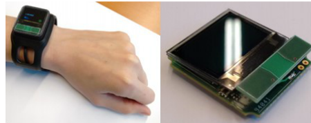
Figure 3. Activity sensor developed in Data-as-a-Service Platform for Healthy Lifestyle and Preventive Medicine (DAPHNE).
