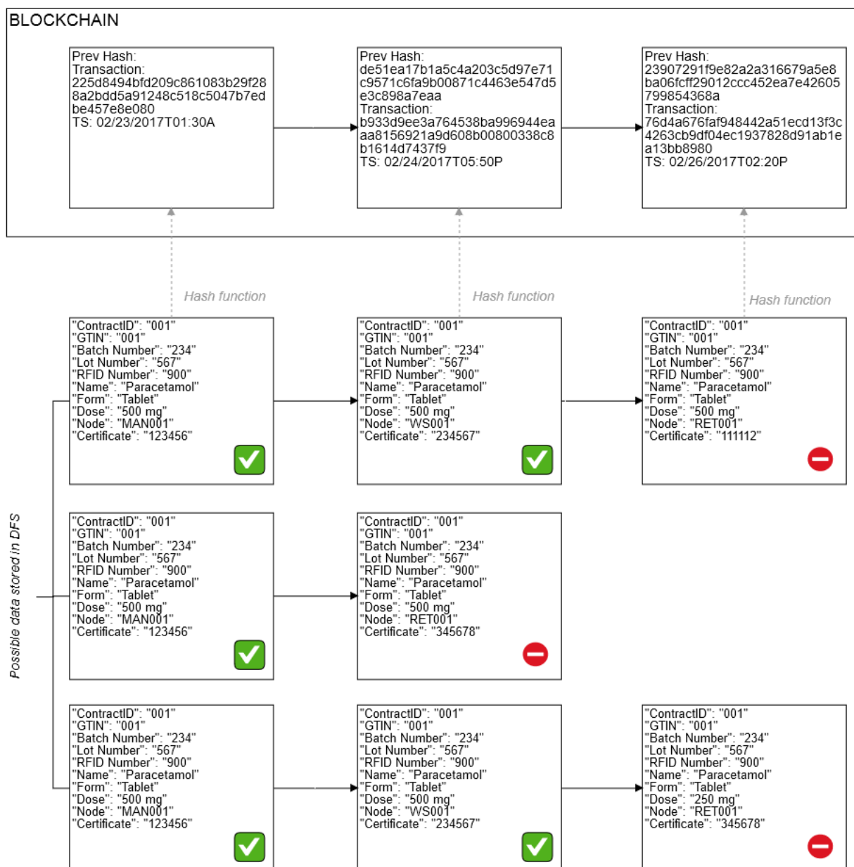
Figure 3. Example of anomalies that can be detected. Top row, information added by a node contains the wrong certificate. Middle row, information is missing from the block. Bottom row, drug product information is different from previous records or does not match the record in the distribution contract registry.
