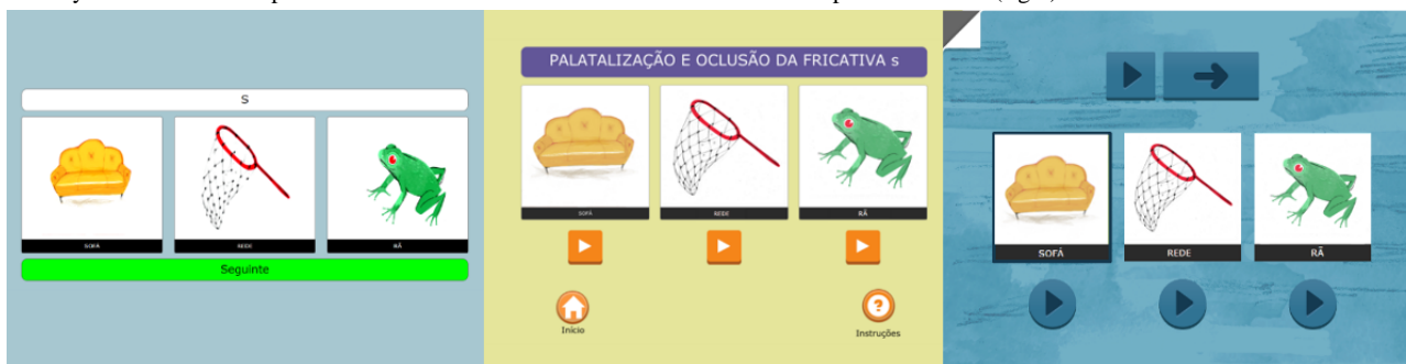
Figure 5. The evolution of the Match activity from the end of second development phase to beta testing. From less buttons and more dependent on the speech and language therapist (left) to less clutter on screen, bigger buttons to accommodate users with less touch screen capacities (middle), and more interactivity in terms of sound production and audiovisual feedback when the user completes an action (right).
