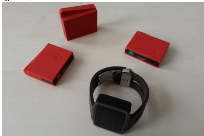
Figure 4. Bluetooth low energy beacon (red) and the sensor bracelet.
