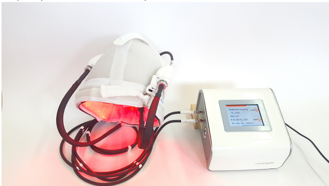
Figure 1. The light-emitting, fabric-based device involved in photodynamic therapy using the phosistos protocol: 635-nm red light is emitted at 1.3 mW/cm 2 by a fiber optic–based fabric that lines the inside of a cap.
