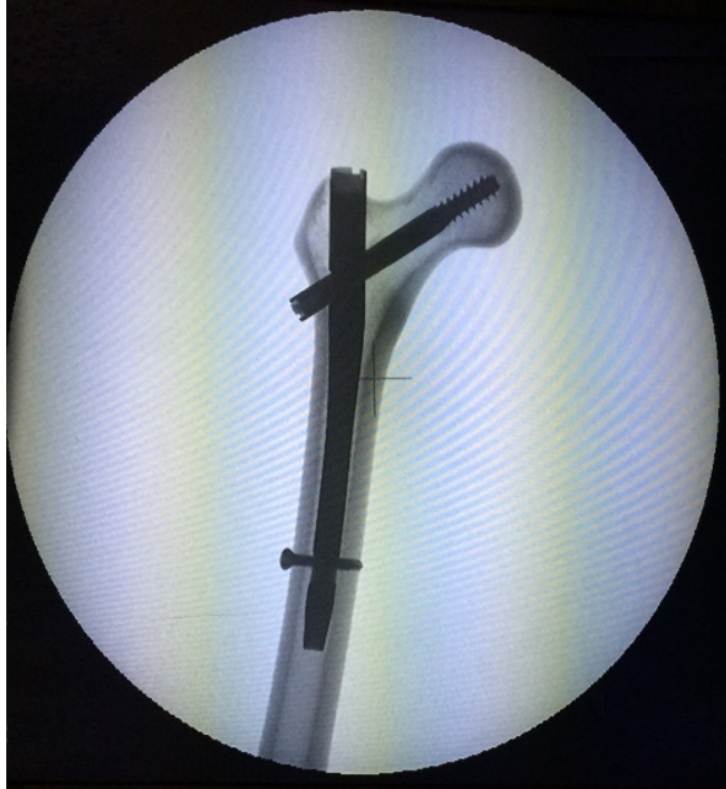
Figure 1. Instrumented Sawbone with Gamma3 nail.
