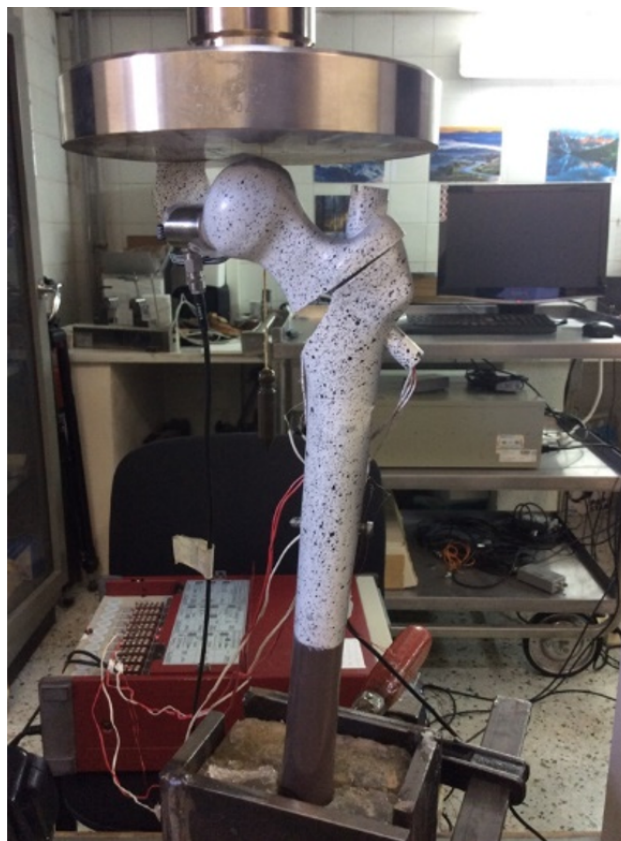
Figure 3. Loading configuration in unstable trochanteric fracture.
