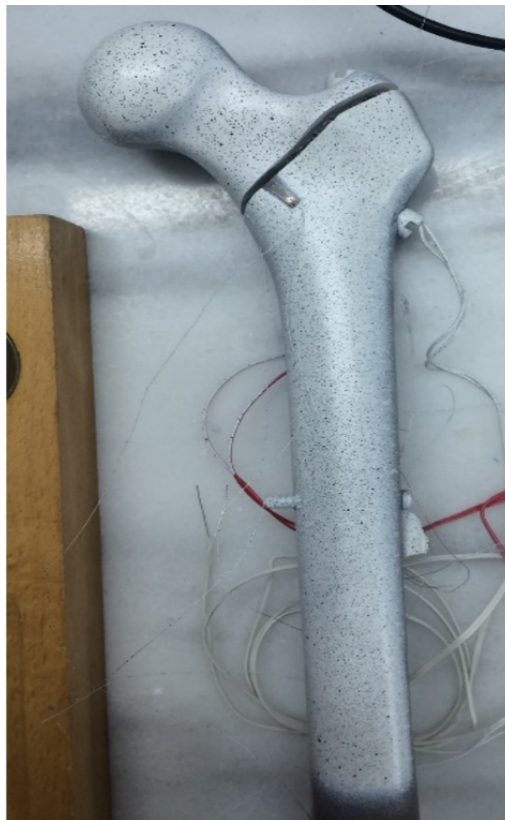
Figure 2. Instrumented stable intertrochanteric fracture with digital image correlation paint and strain gauges.
