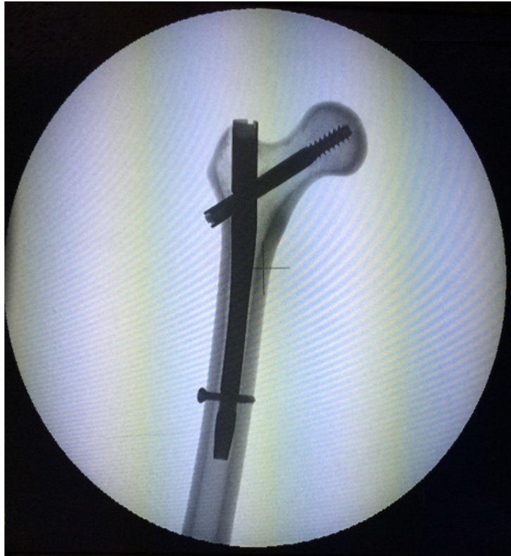
Figure 1. Instrumented Sawbone with Gamma3 nail.
