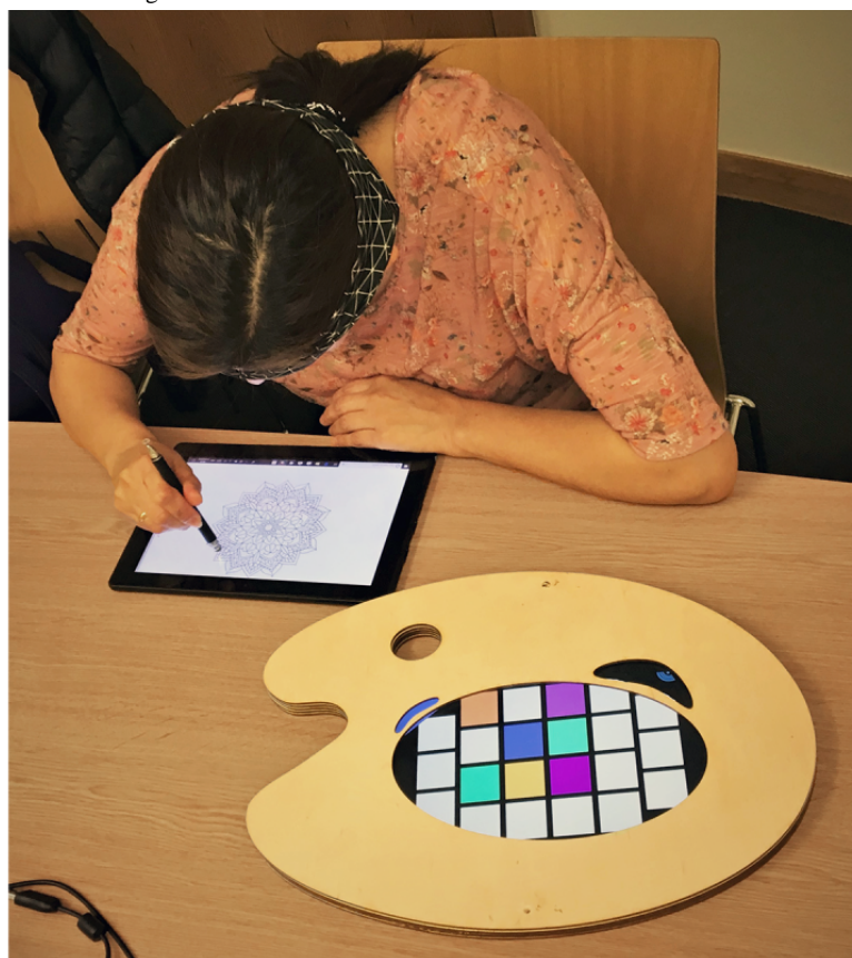
Figure 2. A person using Anima. While wearing the electroencephalography headband, colors based on the current mental states are generated on the wooden palette and can be used to color the digital mandala.
