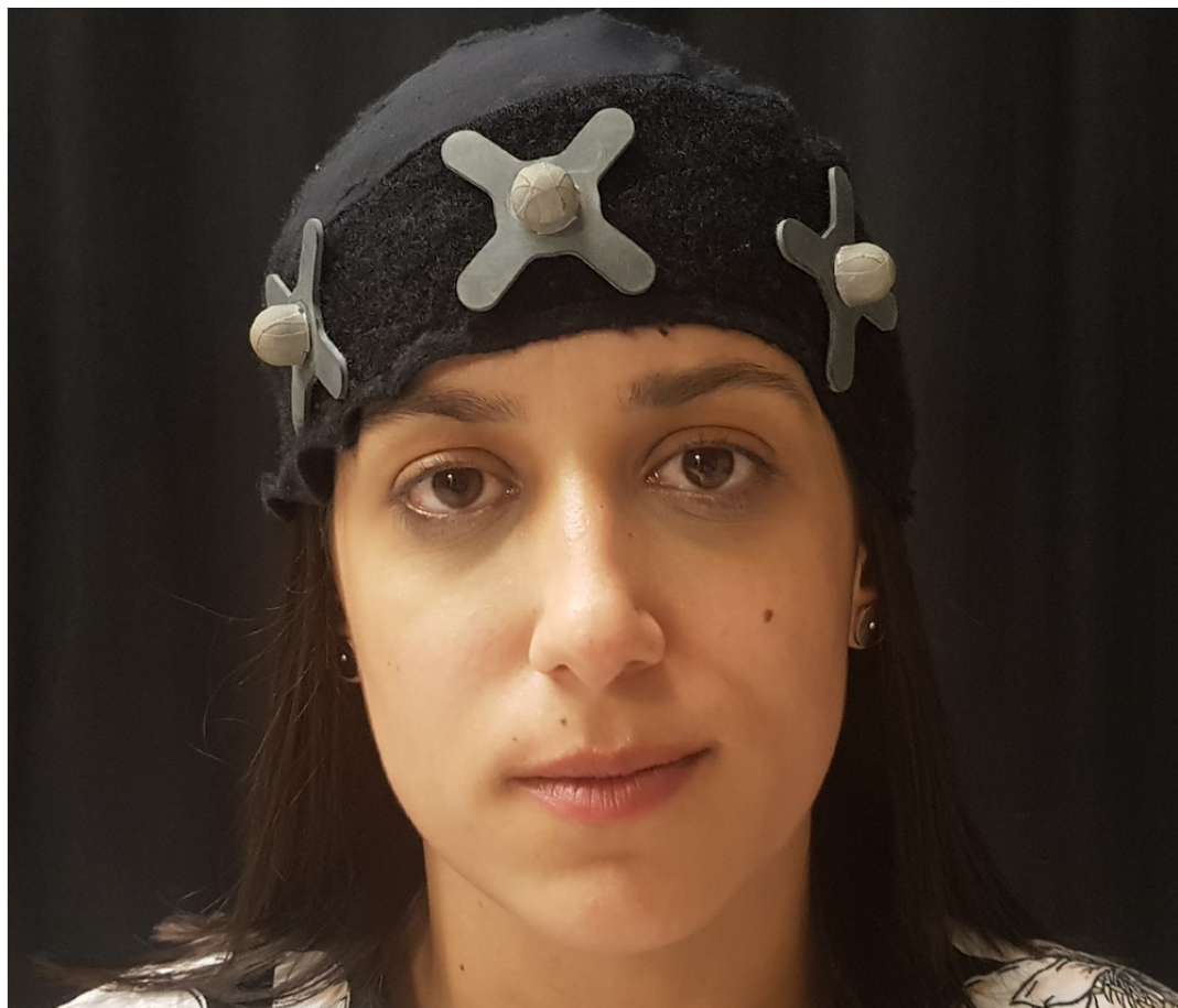
Figure 11. Fabric helmet with sensors for data collection.
