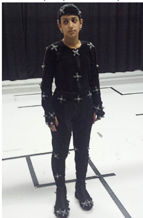
Figure 6. Fabric suits worn by participants on which Motion Capture System sensors were placed.
