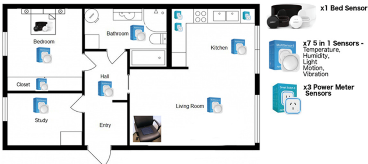
Figure 4. Passive sensors installed in the household to support independent living.
