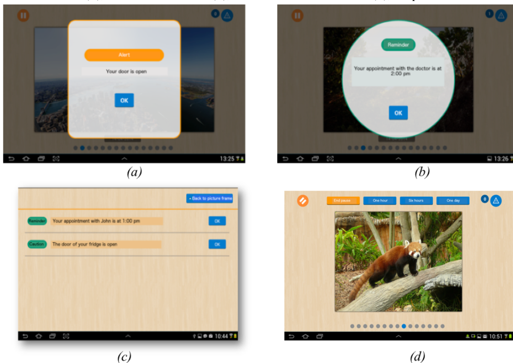
Figure 4. Critical notification (A), noncritical notification (B), list of unattended notifications (C), and pause feature of the notification system (D).
