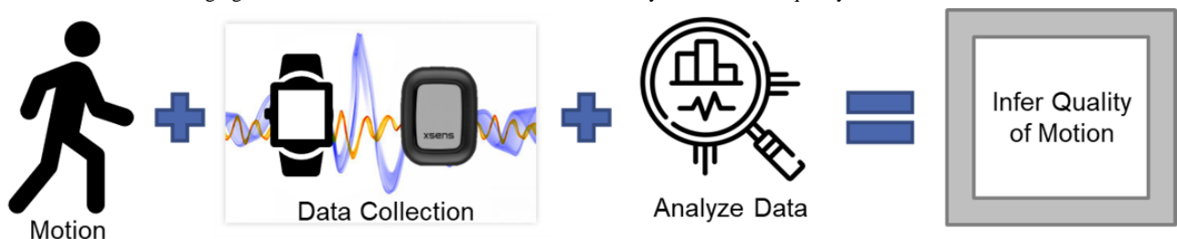
Figure 2. Upper Extremity Examination for Neuromuscular Diseases methodology overview. Participants will perform a set of motions that will be measured via ultrasound imaging and wearable sensors. The data will then be analyzed to infer the quality of motion metrics.
