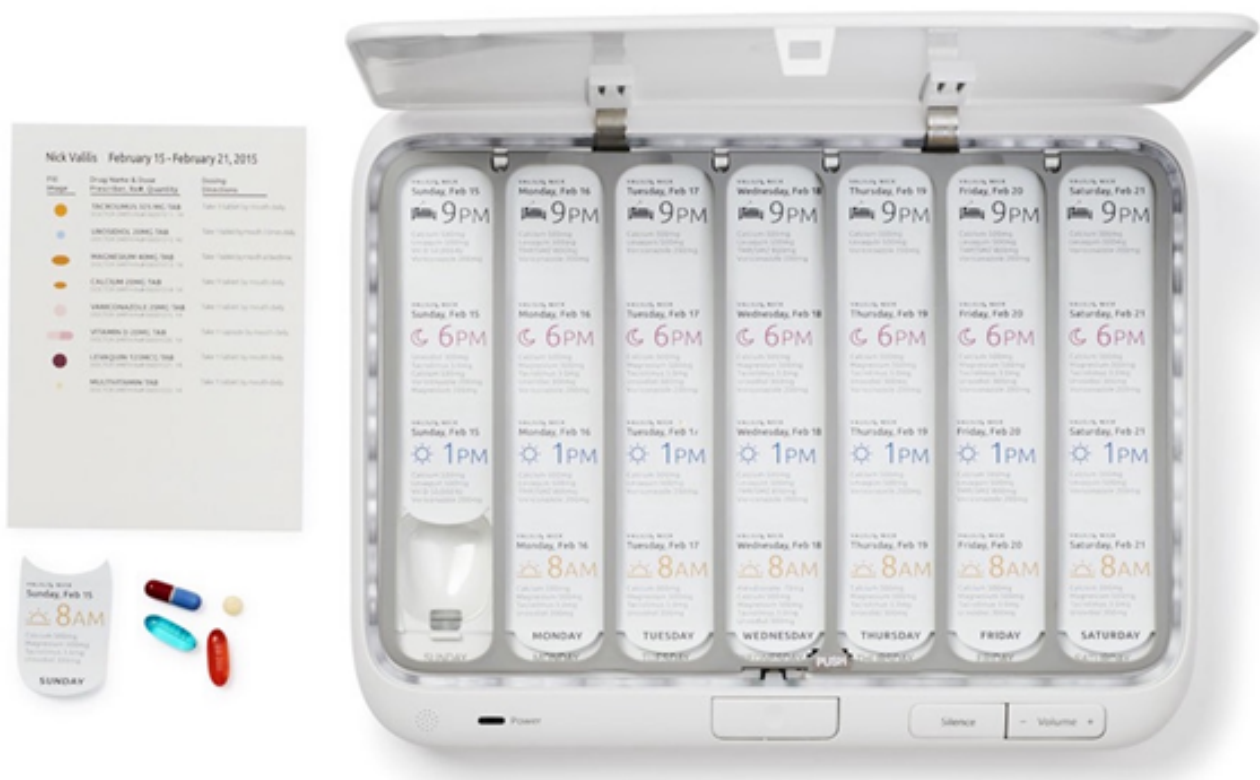
Figure 2. Electronic pillbox TowerView Health used for Project SMART.
