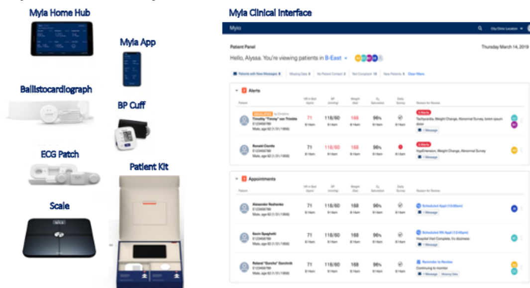
Figure 1. Remote patient monitoring platform used in the Novel Data Collection and Analytics Tools for Remote Patient Monitoring in Heart Failure Trial. BP: blood pressure; ECG: electrocardiogram.
