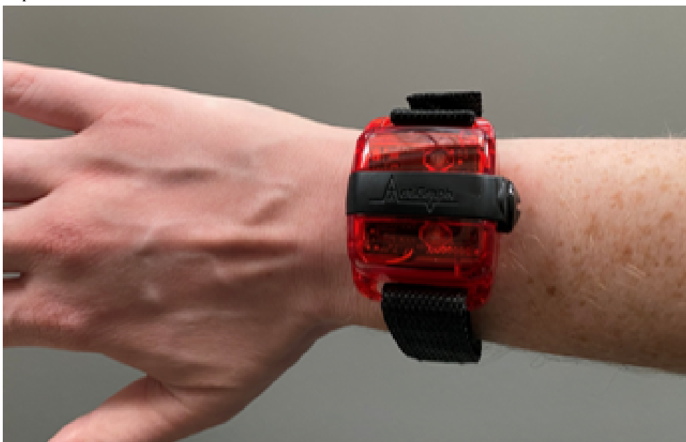
Figure 2. The ActiGraph wGT3X-BT triaxial accelerometer.
